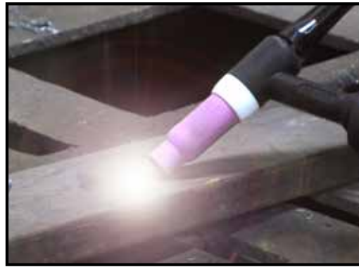
3 The Arc will start forming an arc between the tungsten tip and the work piece
