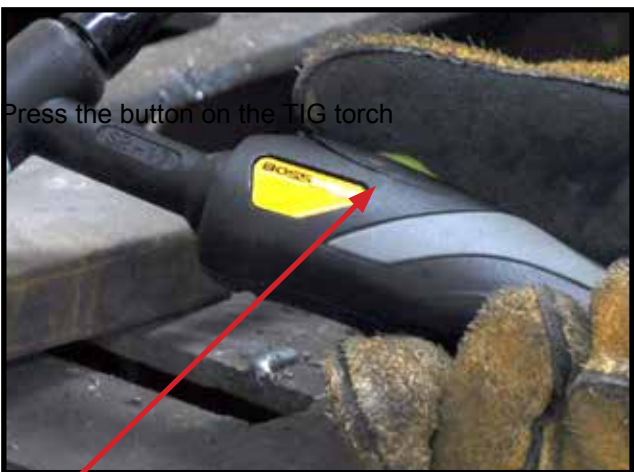
2 Press the button on the TIG torch
