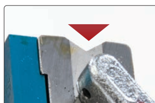
Machined V-Groove For holding round & flat stock.
